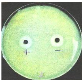
Fig.7 Diameter of E. Coli (1) and hemolytic staphylococcus (2) growth inhibition on the agar under xenoskin in the conditions of disconnected circuit.
